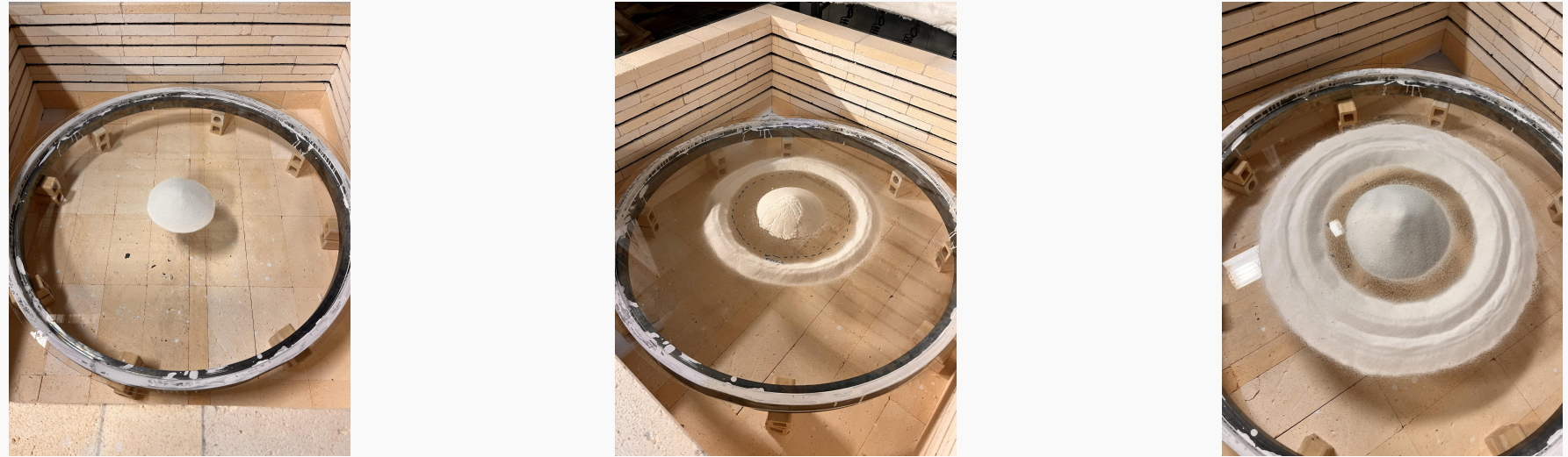
Figure 8: Central Pile(750g), Central Pile(750g) + Single Ring(500g), and Central Pile(1000g) + Multi-Ring (1000g, 500g)
